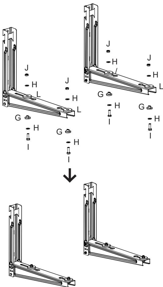
⑥ Monter les plots anti-vibratiles;
